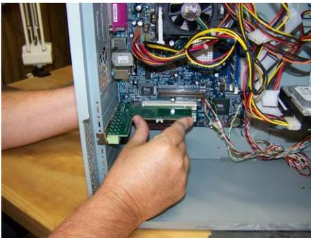
**Support case with hand while pushing card into place.**
