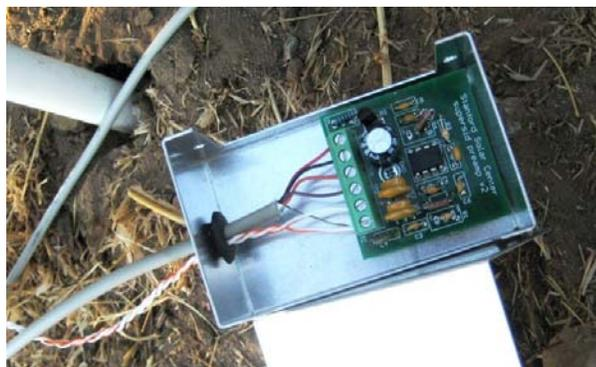
10. Connect the coax cable as described in Chapter 2. Or, if you wish, you can attach the antenna wire (orange/white) directly to the PreAmp.
