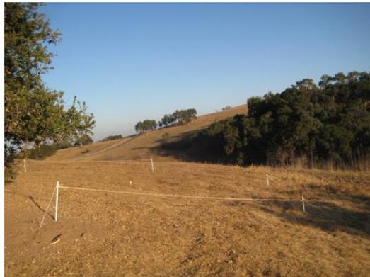
8. To make a hexagonal shape antenna, fold the loop into three, mark 6 segments of equal lengths, and draw a hexagon on the ground.
