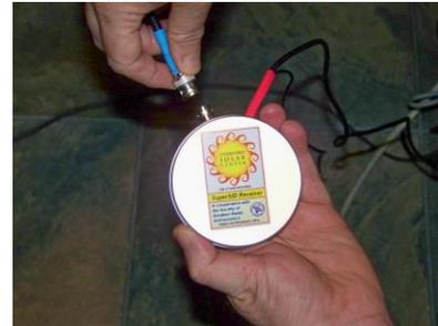
3. Plug the SuperSID cable into the AUDIO INPUT port on your computer.
