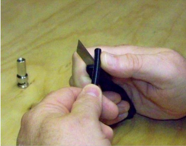
Carefully cut the outer cover of the coax cable.
