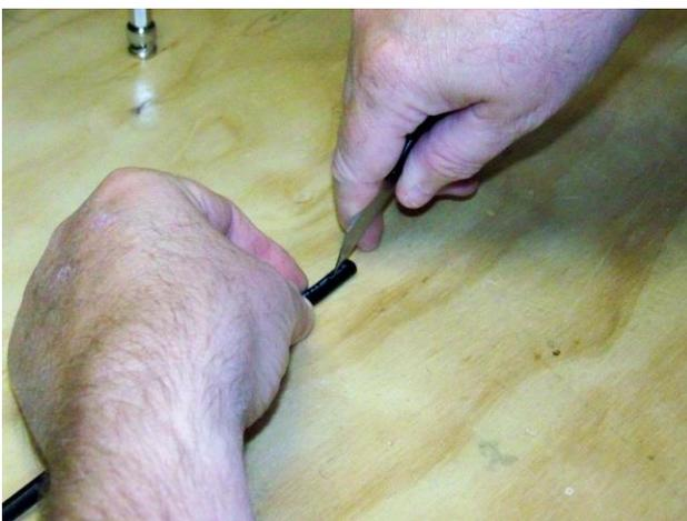
From the first cut around the cable, take the knife and cut a line to the end of the cable.
